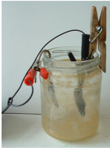
N.B. I use a clothes peg to make sure the electrodes are kept separate
